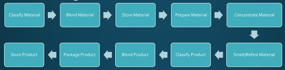
Ore Processing focuses on the following procedures:
